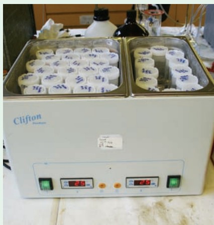
Water bath containing individual steel samples in pond water solutions, held at constant temperature.
