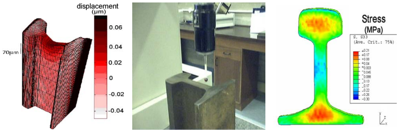
The surface profile (exaggerated) of the cut surface as determined by CMM (left) The inferred longitudinal stresses prior to the cut (right)
